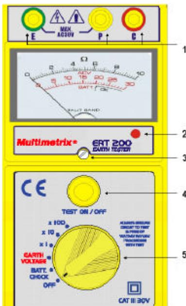
1 - bornes de raccordement E (Terre), P (Potentiel), C (Courant)
