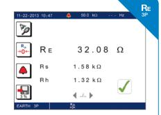
3-pole earth measurement using 2 auxiliary stakes (also known as the 62 % method) is the earth measurement of reference which yields a precise resistance value for the earth electrode.
