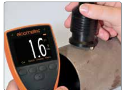
Integral or separate probes measure profiles up to 500μm (20mils) on flat or curved surfaces**
