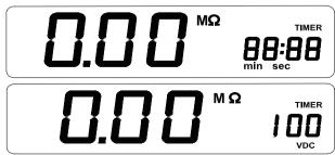
Press SELECT to check the preset time. The LCD screen display TIMER, PRES is shown on primary display, the secondary display shows the preset time. Press ENTER, the meter display Set. The time can be adjusted by  $\triangle/\nabla$  button.
