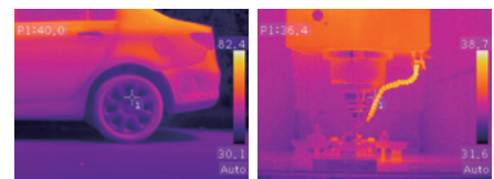
Auto Fusion mode (AUF) A dynamic image enhancement-algorithm for infrared cameras
