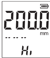
High alarm limit setting.
